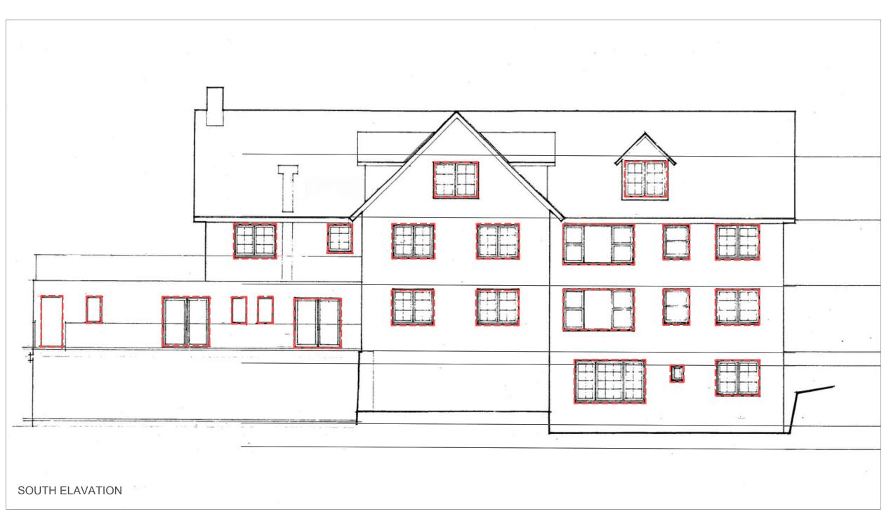
existing timber windows are to be replaced with double glazed aluminium windows with matching fenestration (pane size etc.) - Openable portions of window to have fixed metal screens meeting requirements of clause D2.24 of BCA (NCC Vol. 1)
