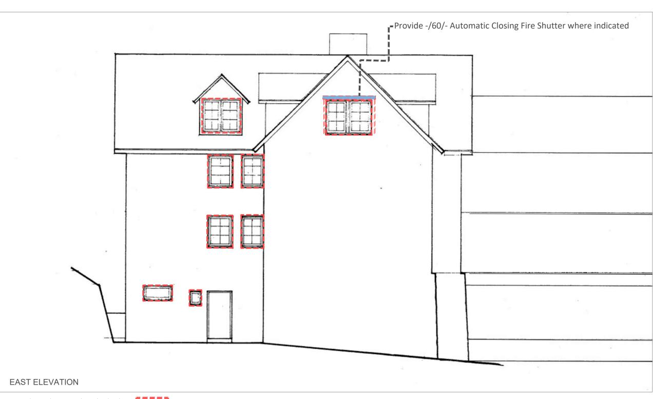
existing timber windows are to be replaced with double glazed aluminium windows with matching fenestration (pane size etc.) - Openable portions of window to have fixed metal screens meeting requirements of clause D2.24 of BCA (NCC Vol. 1)
